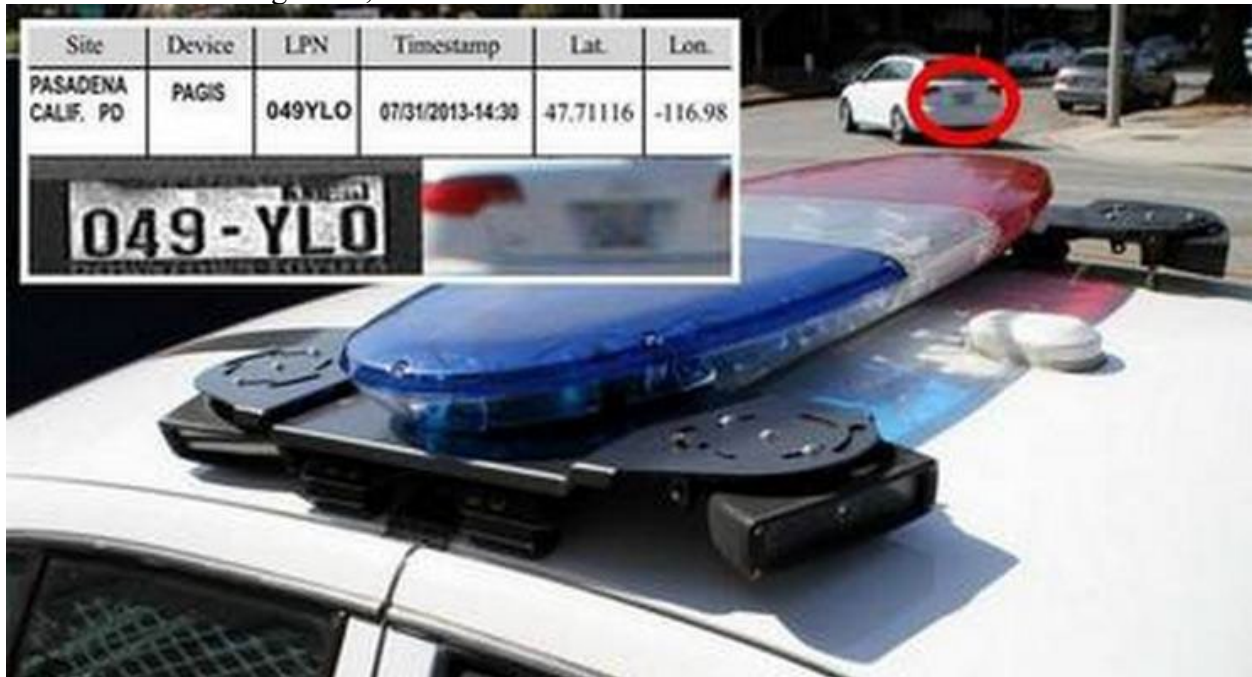
Figure 1: Police vehicle with an Automated License Plate Reader mounted on its roof, and an example picture from the ALPR camera (top-left). This ALPR picture identifies 1) the license plate, 2) the time and location of the car, and 3) other information captured in the photograph, including vehicle color, make, and model. Source: Pasadena, CA Police Department.
